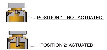
Before threading the Cable-operated manual actuator to the activation port of the valve, check that the actuator pointer is retracted (position 1).
