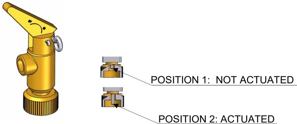
Before threading the pneumatic manual actuator to the activation port of the valve, check that the actuator pointer is retracted (position 1).
